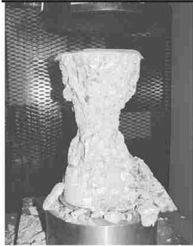
Fig. 4.6 Concrete specimen failed in compression test. [NRMCA, 2003]
